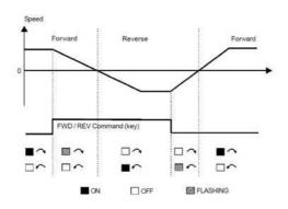
Figure 5.2 - Direction of Rotation (FWD / REV) LEDs
