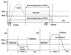
Figure 6.8 - Actuation levels for over and undercurrent
