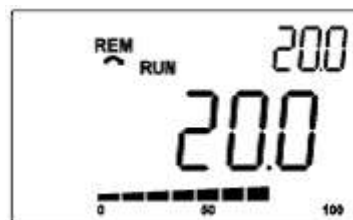
Figure 19.21: Example of HMI in the monitoring mode for the PID2 Controller function
