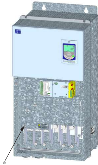
Figure A.4: Location of filter capacitors ground disconnection points - disconnection trough bolts - frame sizes F and G
