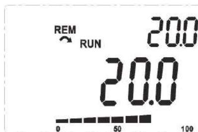
Figure 15.3: Example of HMI in the monitoring mode to use the PID controller
