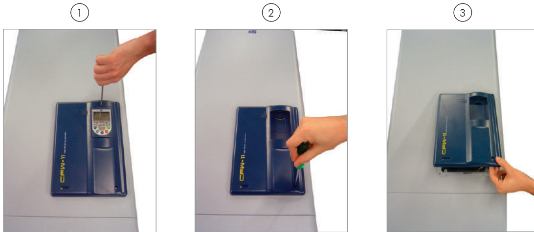
Figure 3.3 - Removal of the HMI and the control rack cover
