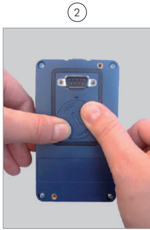
Press the cover and rotate it counterclockwise
