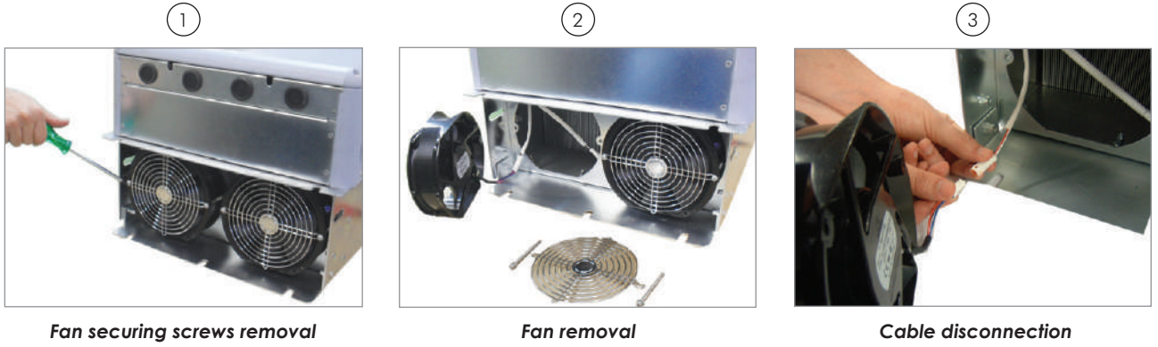
Figure 6.1 - Removal of the heatsink fans
