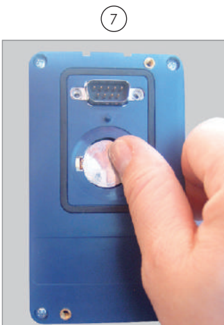
Press the battery for its insertion
