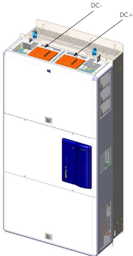
(d) Frame size G with special DC hardware: Terminals for DC voltage supply. Terminals R/L1, S/L2 and T/L3 are not internally connected in this version
