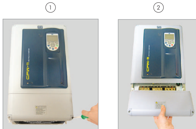
Figure 3.7 - Bottom front cover removal
