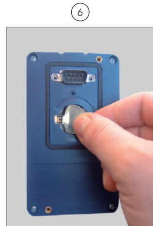
Install the new battery positioning it first at the left side
