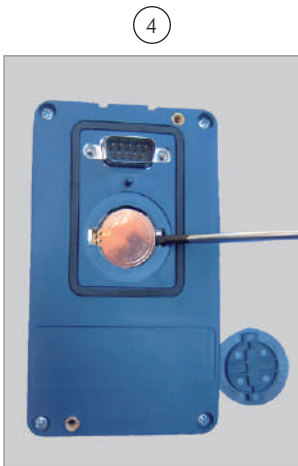
Remove the battery with the help of a screwdriver positioned in the right side
