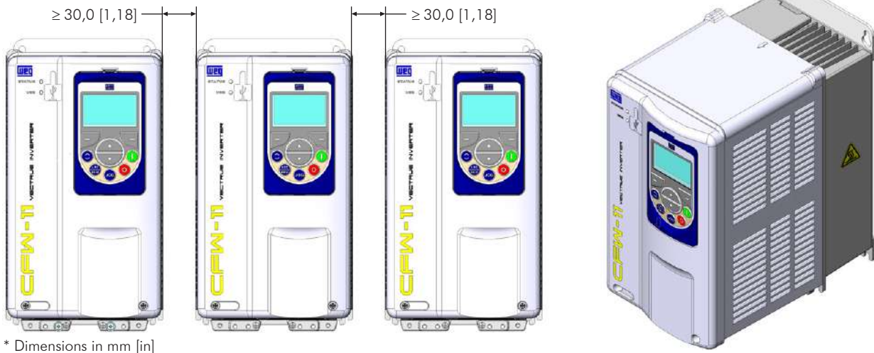
(a) Minimum side clearance requirements
