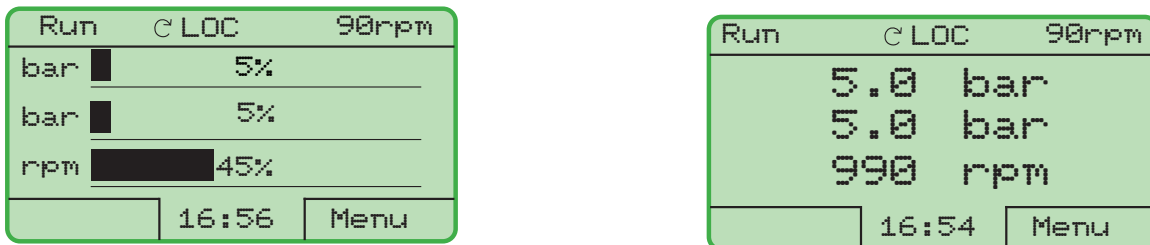
Figure 20.4 - Example of the keypad (HMI) in the monitoring mode for the PID Regulator function
